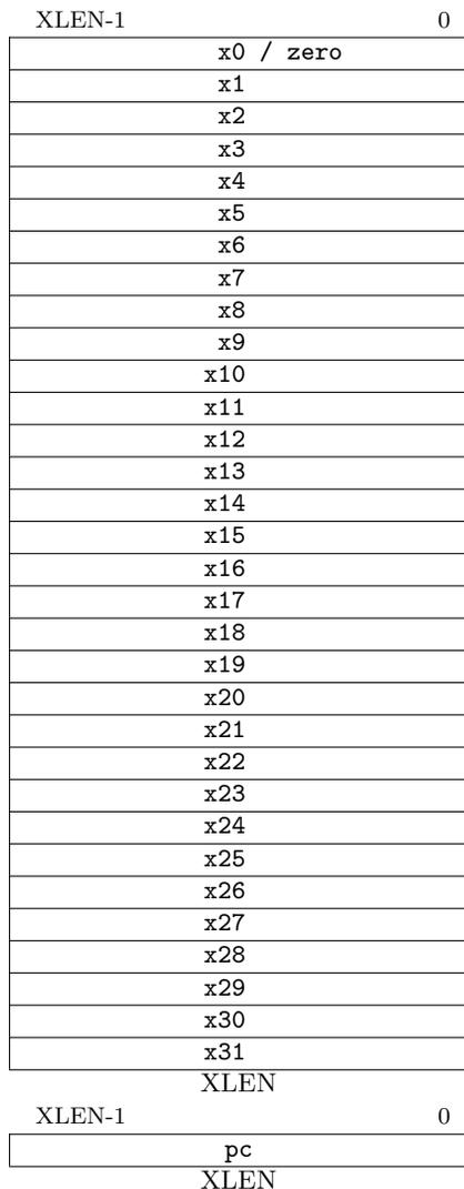
Figure 2.1: RISC-V user-level base integer register state.
