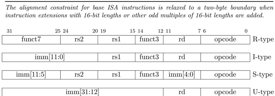
Figure 2.2: RISC-V base instruction formats. Each immediate subfield is labeled with the bit position ( $\text{imm}[x]$ ) in the immediate value being produced, rather than the bit position within the instruction’s immediate field as is usually done.
